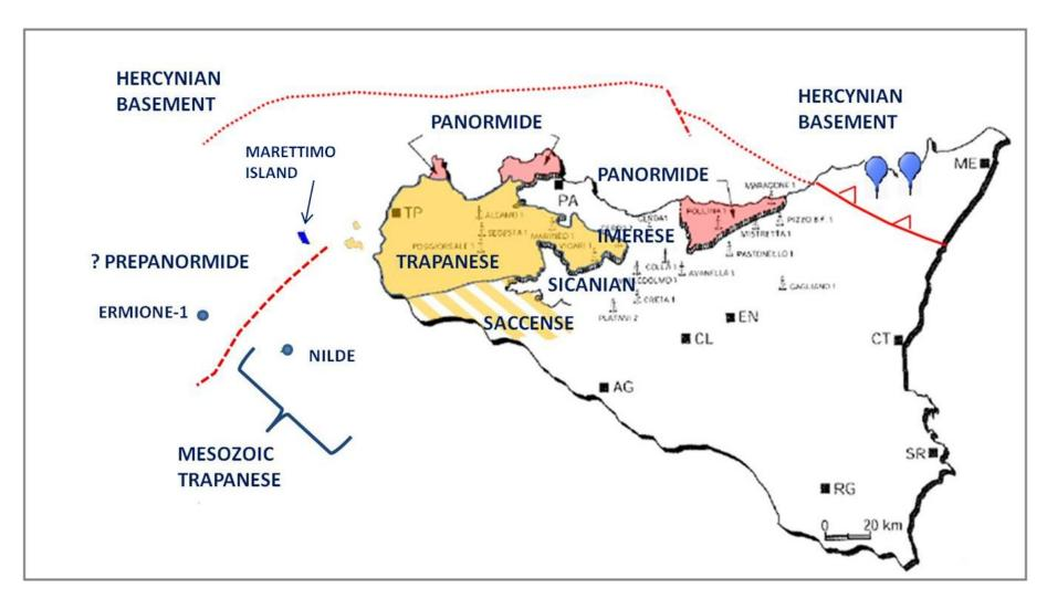
Figure 5. Tectonic map of Sicily representing the main paleogeographical units in the onshore/offshore thrust belt (modified after G. Miuccio et al., 2000). Thick platform units in the onshore thrust belt (reached by wells and outcrops) are in colour, allochthonous units are indicated but left blank. Blue place marks in north-eastern Sicily refer to Late Cretaceous organic rich samples from Novara di Sicilia and Floresta.
