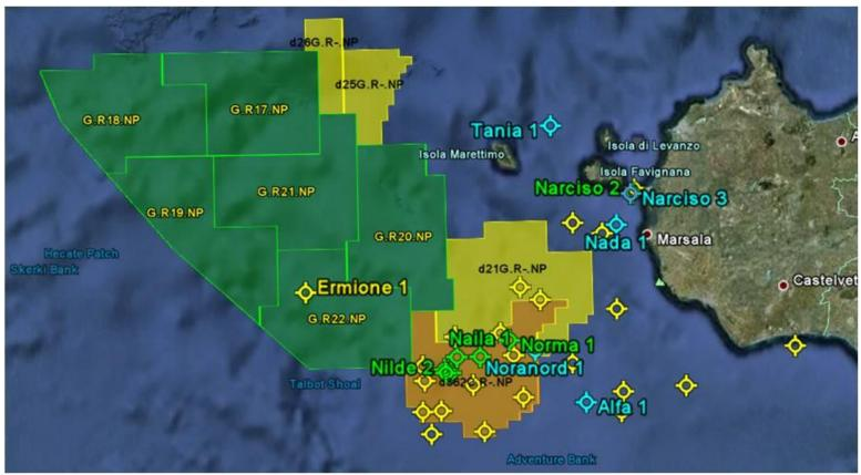
Figure 2. Offshore thrust belt well database and Northern Petroleum (NP) permit areas. Drilled wells: green indicates discoveries, in yellow are dry wells, blue indicates wells which had oil or bitumen shows. NP permit area: green polygons indicate NP awarded permits, yellow polygons are NP applications, orange polygons are NP contested applications. (Image from Google Earth).
